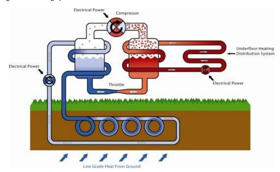
Fig 1. Heat pump Schematic
