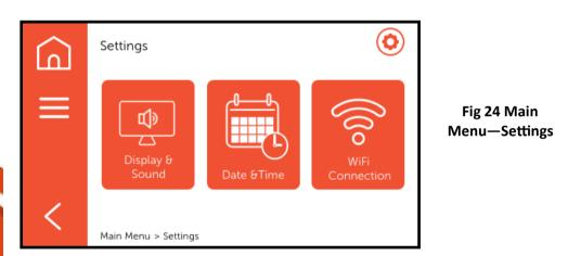
The settings screen allows some customisation of the controller. This includes the wi-fi set up and date and time. If the Wi-Fi symbol is not shown then the heat pump is not internet ready.
