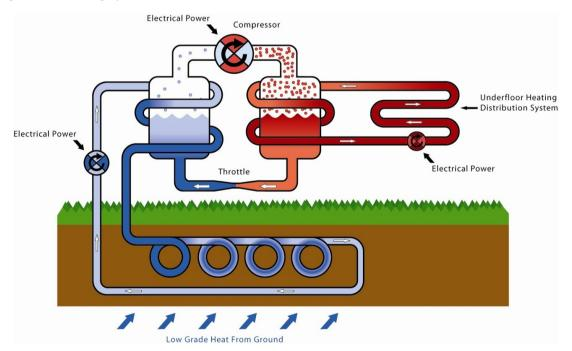
Fig 1. Heat pump Schematic
