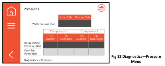
The pressure screen shows the current pressures measured within the system.
