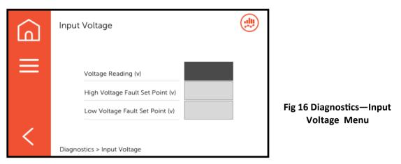
This screen indicates the measured voltage connected to the heat pump. It is an indication of the approximate voltage with a tolerance of +/-10%. It also indicates the voltage at which a fault is indicated and registered.
