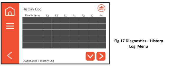
The history log records various readings from the heat pump every 15 minutes. It stores data over the last 37hours and is a useful tool to help with intermittent fault finding. The unit itself holds data further back which can be accessed only by a Kensa Engineer.
